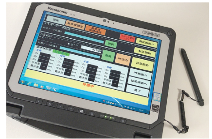
The tablet PC that controls the Mobile 3D Tunnel Scanning System
