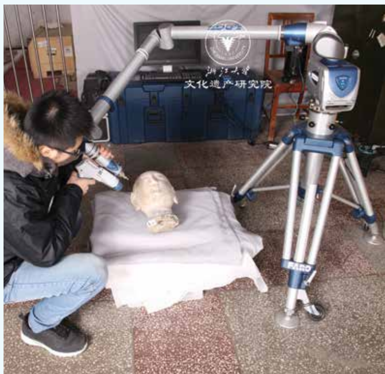
A team member uses the FARO ScanArm to perform scans on stone steles in the Xi'an Forest of Stone Steles Project.
