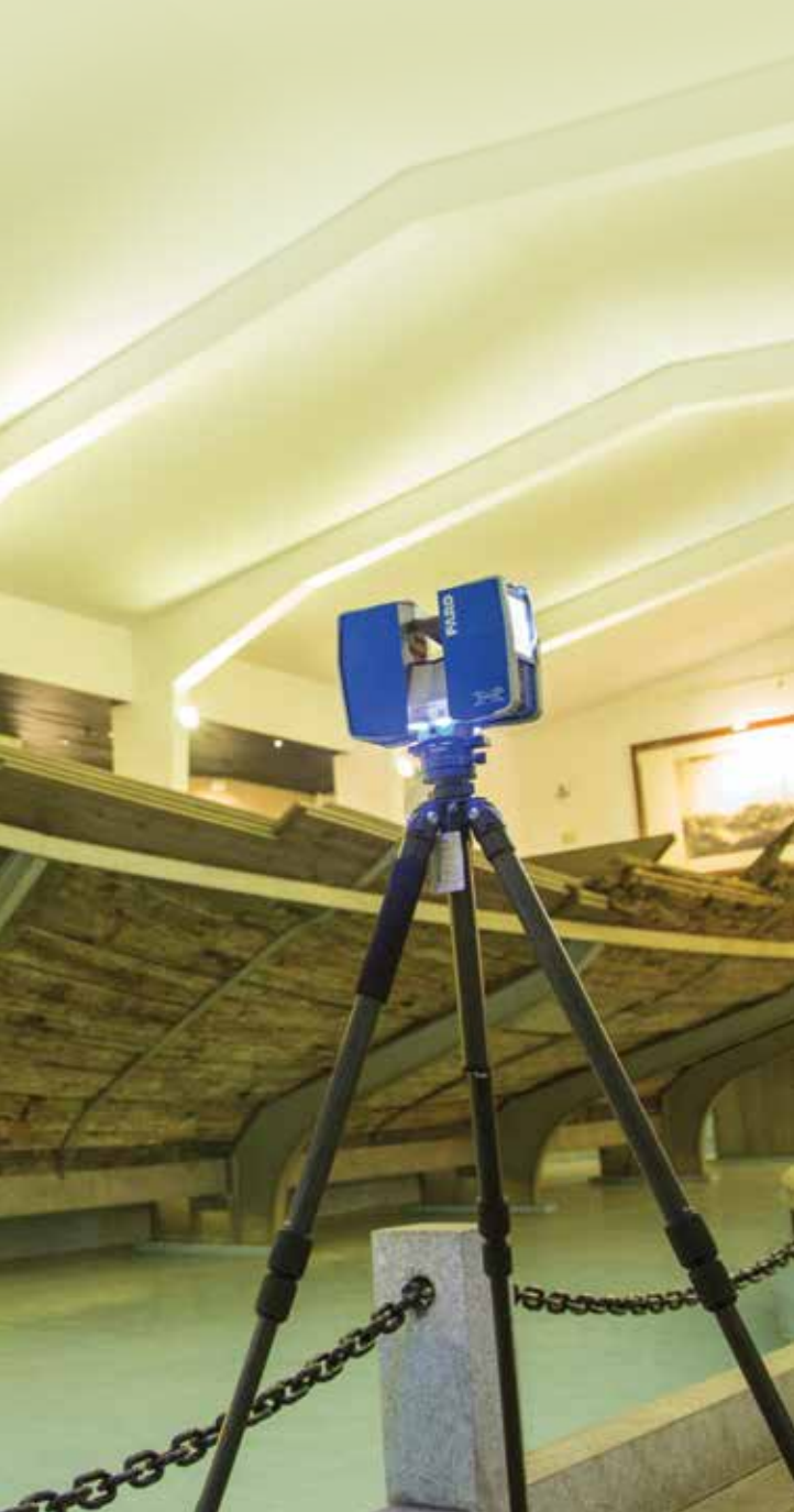
Obtaining measurements of the Seventh Cave in the Eastern Thousand Buddha Caves with 3D laser scanning.
