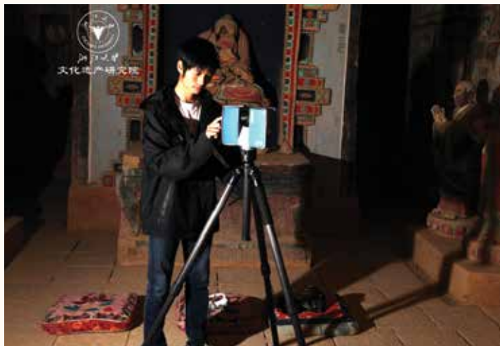
Obtaining measurements of the Seventh Cave in the Eastern Thousand Buddha Caves with 3D laser scanning.
