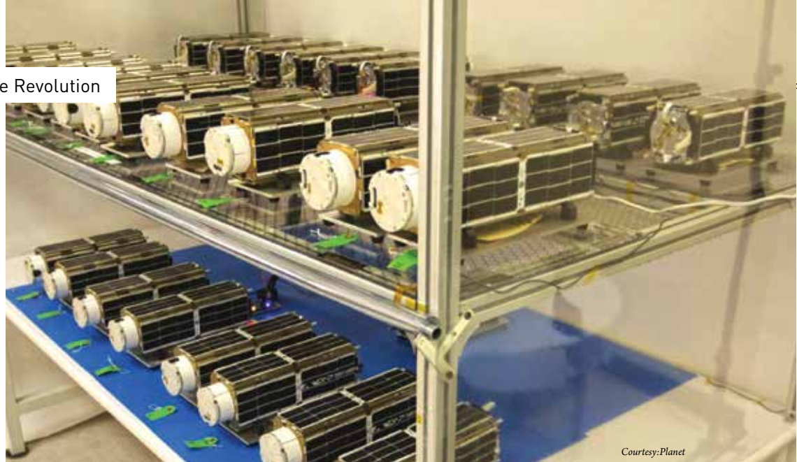
Planet's Doves weigh about 5 kg each, and are designed and built in-house
