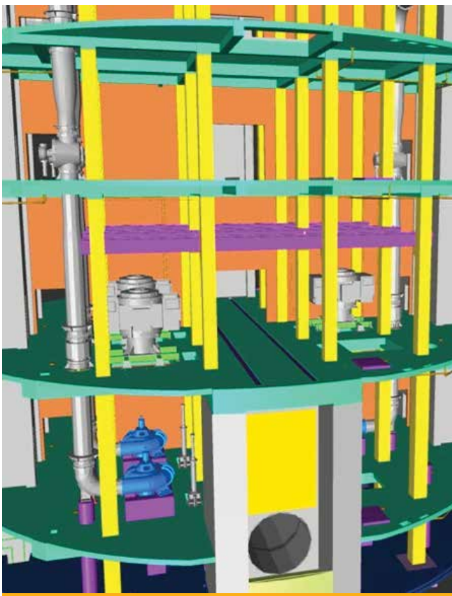
»» The lower levels of the pumping station model. The pipe opening on the lower level is 13 feet (4 m) in diameter.
